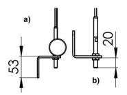
Lower brackets can be installed on the side or front, while the angle section aims down (a) or up (b).
