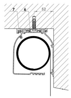
Attach brackets (6) using components screws and suitable the for type structure onto which they are be attached (metallic structure, window frame, wall, other material). If four brackets are used, ensure that the brackets are perfectly aligned ± 1 mm; this can be checked by sliding the box along the cut-outs before tightening the attachment screws.
