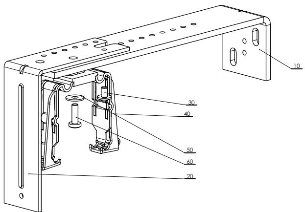
Support reglable - mecanique 306 – 368 mm
